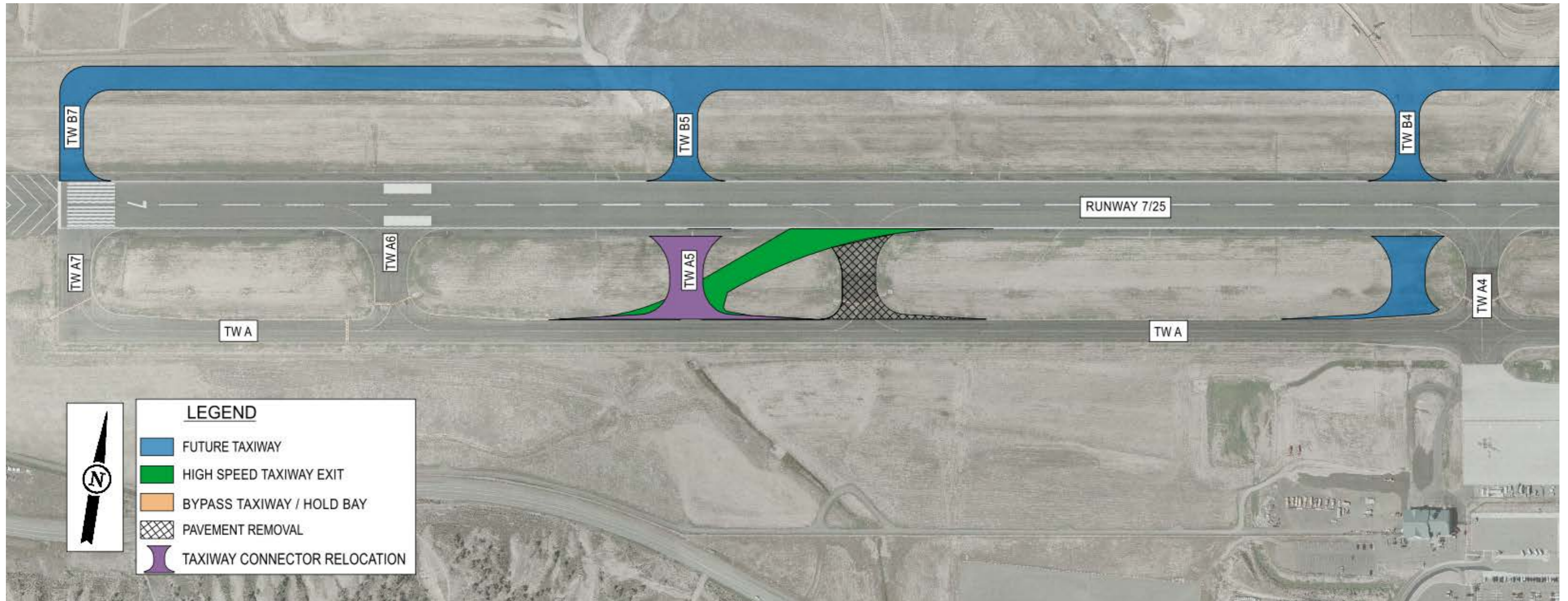
FIGURE 5-8 – HIGH SPEED TAXIWAY EXIT
